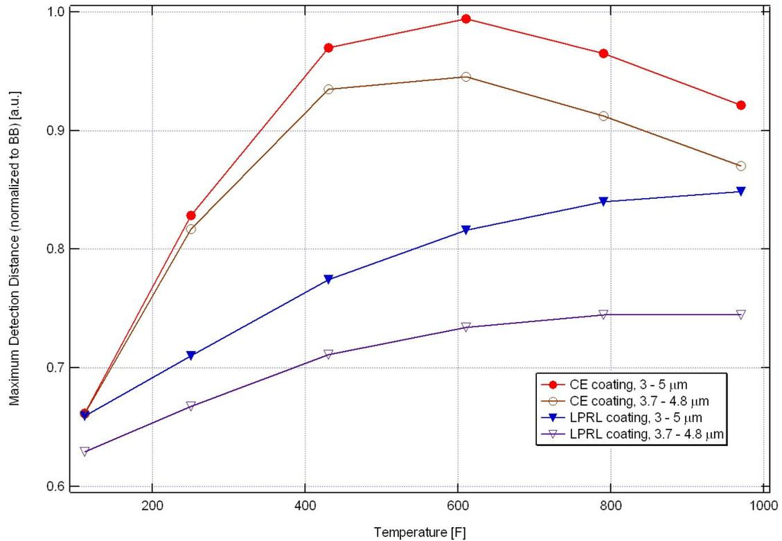
**Figure 5: The maximum detection distance for the heated cubic centimeter black body coated with the LPRL coating (blue curve) and the constant emissivity (CE) coating (red curve). Both curves are normalized to the maximum detection distance of the black body cube (see Equation 7). For each coating, we show the result for band II (3 to 5  $\mu\text{m}$ ), and for the portion of the band detected by most IR detectors (3.7 to 4.8  $\mu\text{m}$ ).**
